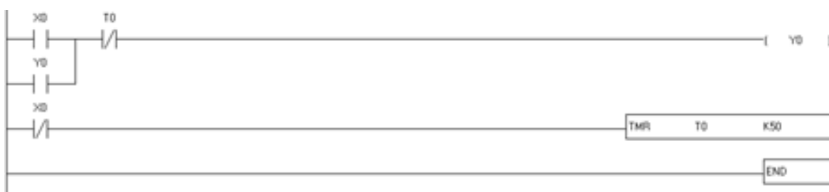
Figure 14.3 PLC Ladder Diagram for OFF Delay Timer
