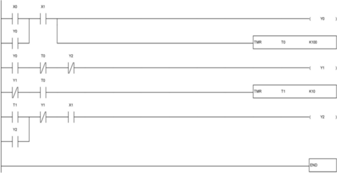
Figure 2.3 Star-Delta starter ladder diagram
